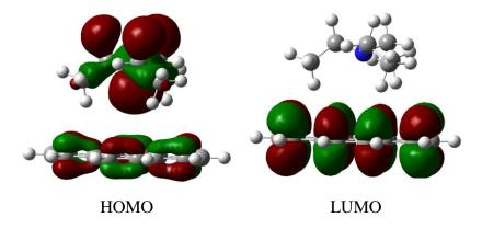
Analyses of first excited singlet states have revealed that there are charge transfers between Pyrene and investigated amines. Figure shows charge transfer between Pyrene (Py) and trimethylamine (TEA) in gas phase.  $S_0 \rightarrow S_1$  transition (376 nm) between H $\rightarrow$ L orbitals for Py-TEA system has a CT character from TEA to Py.
